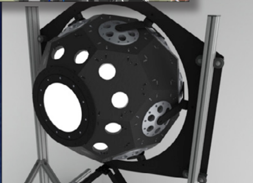
26 in Geodesic Spectralon SIRCUS (Laser) Calibration Sphere for NASA
