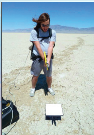
Classic Spectralon Target for Spectral Ground Truth Reflectance
